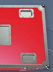
Featuring a 9mm plywood carcass, with a smart High-Pressure Laminate (HPL) exterior finish and high quality Penn Elcom hardware. 30mm aluminium angle and mating location profiles to all exposed edges. 4" heavy-duty casters are fitted as standard, two of which are braked.
