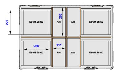
E8 with Z5350 Length: 232mm Width: 223mm Height: 390mm
