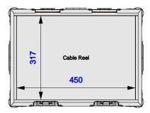
Cable Reel Length: 445mm Width: 312mm Height: 555mm
